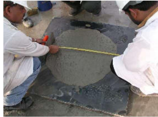
Figure 10 – SCC Conc. Flow Table Testing
