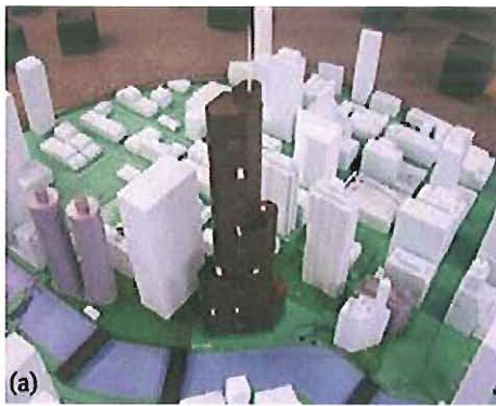
Fig. 5: Wind tunnel studies were used to evaluate the building's dynamic response: a) an aeroelastic model of the tower was mounted among scale models of existing buildings; b) models were mounted on a carousel so that wind direction could be varied; and c) the partially assembled model shows the sophisticated fabrication required for aeroelastic modeling (Photos courtesy of Rowan Williams Davies & Irwin, Inc.)
