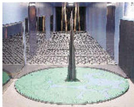
Figure 14 – Aeroelastic Wind Tunnel Model (Image courtesy of RWDI)
