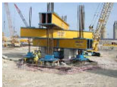
Figure 12 – Test Pile (6,000 tonnes)
