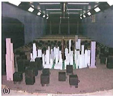
Fig. 5: Wind tunnel studies were used to evaluate the building's dynamic response: a) an aeroelastic model of the tower was mounted among scale models of existing buildings; b) models were mounted on a carousel so that wind direction could be varied; and c) the partially assembled model shows the sophisticated fabrication required for aeroelastic modeling (Photos courtesy of Rowan Williams Davies & Irwin, Inc.)
