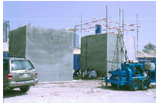
Figure 11 – Raft Conc. Placement Test Cubes
